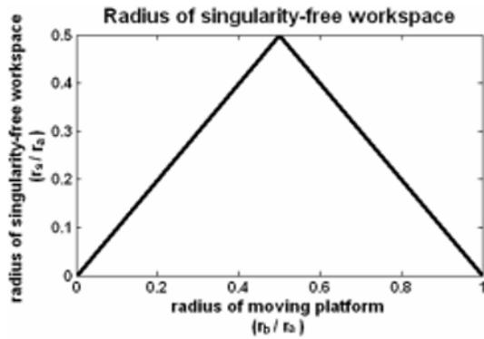
Fig. 5. Radius of the singularity-free workspace along the radius of moving platform ( $r_b/r_a$ ).
