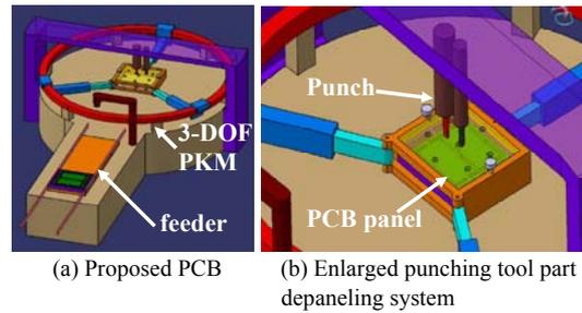
Fig. 6. Conceptual design of the PCB depaneling machine using the planar parallel mechanism and a punching tool.
