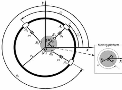
Fig. 3. Description of the mechanism and kinematic parameters.
