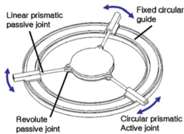
Fig. 1. Architecture of the novel 3-DOF planar mechanism.
