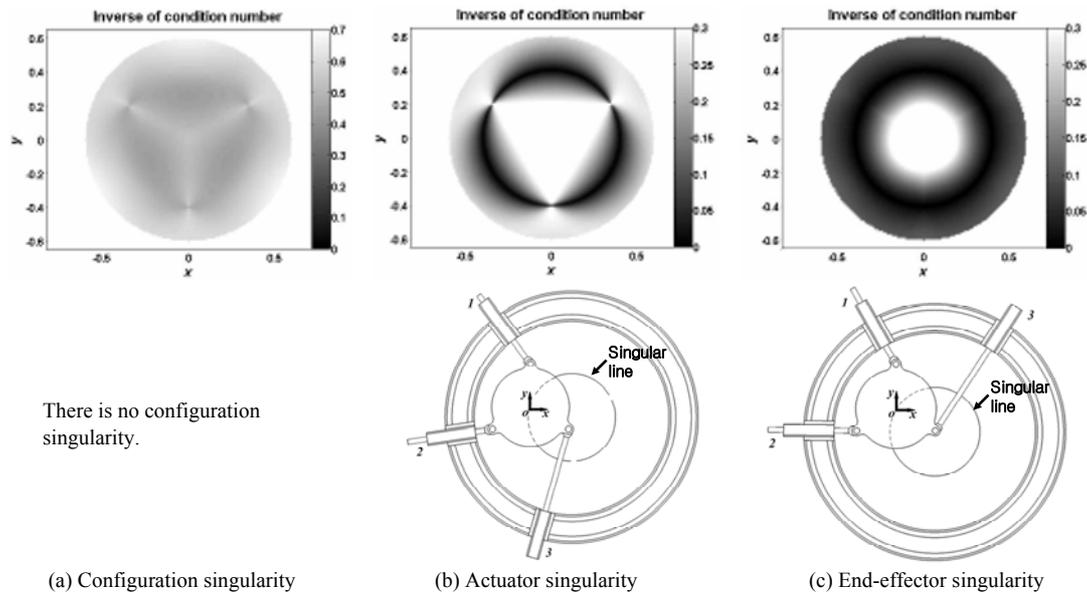
Fig. 4. Singularity analysis using the inverse of the condition number and an example of a singular configuration.
